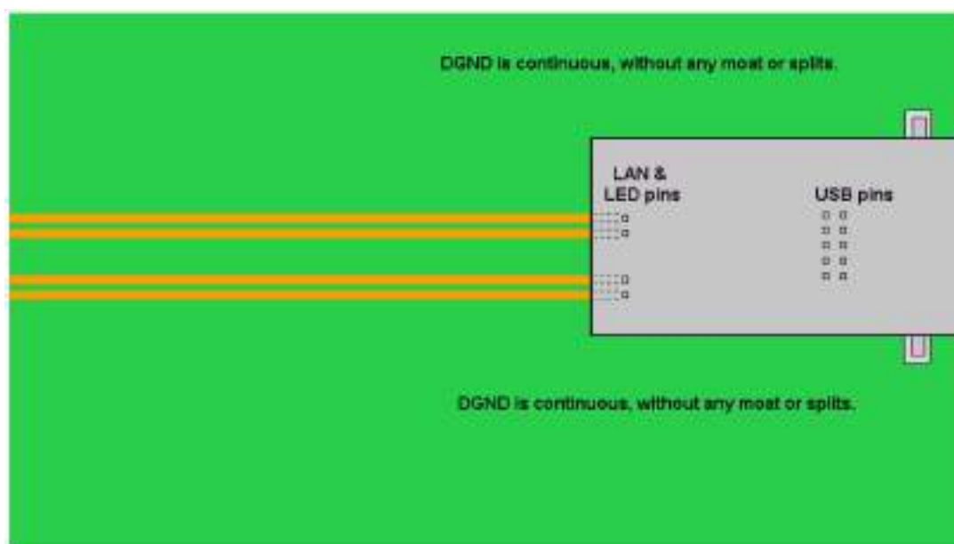
Figure 13-19 Ground Layout with USB
